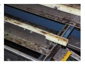
Although the roller cable carriers have been in operation for over two years, they so far show no sign of wear whatsoever. The cable carrier systems are tested every month, after which a test report is generated. These reports confirm that no abrasive wear has taken place to date.
